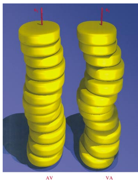
Figure 3. The channel shape in AV (left) and VA (right) shown as a set of inscribed disks threaded on a sixfold screw axis. Two c -translation periods are shown for each dipeptide.
